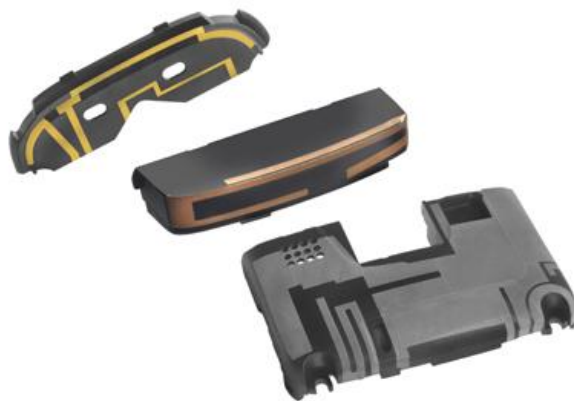
Antenna carriers made from XANTAR LDS (picture name JOZ0053)
